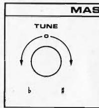
MASTER TUNE is the overall tuning control for the entire instrument over a narrow (+/- minor 3rd) span. Use this control to match the pitch level of the Spirit to other instruments. (Although this control affects both oscillators equally, tune by listening exclusively to Oscillator A, since Oscillator B might be detuned widely due to its INTERVAL control setting. After tuning while listening to Oscillator A, tune Oscillator B to match A, or to desired interval above or below A.)
