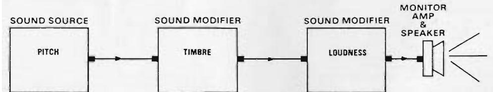
The path from sound source through the modifiers to the speaker is called the "audio signal path." Note that the sound source has only an audio output since it actually generates the audio signal. The modifiers have both an audio input and an audio output since the signal to be modified passes through them.
