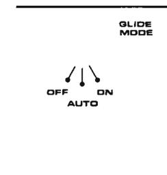
The GLIDE MODE switch offers a choice of OFF (no glide), AUTO (glide occurs only when more than one key is depressed, allowing you to introduce glide selectively from the keyboard), and ON (glide on all the time, regardless of keyboard technique).
