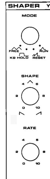
SHAPER Y controls determine shaper output symmetry and rate, and response to keyboard gates.
