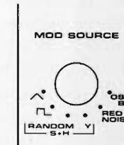
The MOD SOURCE SELECTOR selects one of six possible modulation types: LFO triangle wave; LFO square wave; S + H RANDOM (red noise sampled); S+ H Y (Shaper Y signal sampled); RED NOISE (continuous red noise random signal); and OSC B (triangle wave output). The selected signal is always routed to the MOD X wheel to the left of the keyboard, where modulation amount is controlled.
