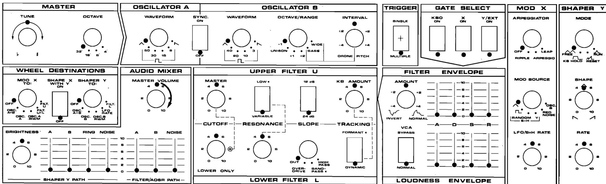
Rotary pots to 12 o'clock. Rotary switches to left. Rocker switches down. Sliders down.
