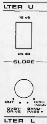
The LOWER FILTER SLOPE switch is most important in filter mode selection on the Spirit. Its positions provide filter responses as follows:
