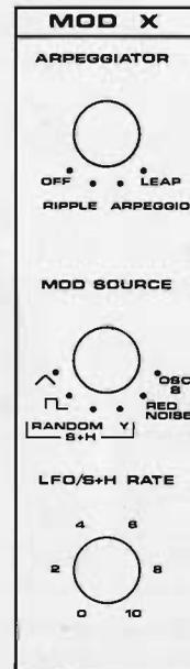
MOD X controls determine modulation shape and rate of LFO (low frequency oscillator) sources, permit selection among keyboard arpeggiation modes, and selection of other modulation sources.
