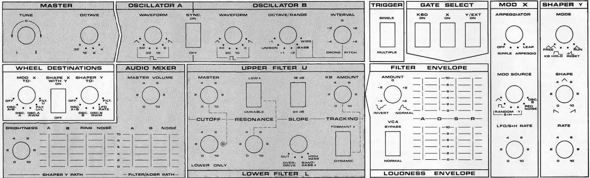
The Sound Sources of the Spirit include two tone oscillators and a noise generator. The Noise signal is a combination of white and pink random noise suitable for producing pitchless sounds. A ring modulator provides clangorous (bell-like) sounds by generating new partials (sum and difference pitches) from OSCILLATOR A&B triangle waveforms via fixed internal connections.
