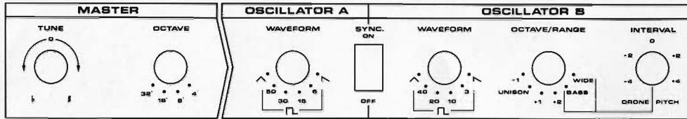
Oscillator controls are divided into a MASTER section that affects both oscillators, and individual OSCILLATOR A and OSCILLATOR B sections.
