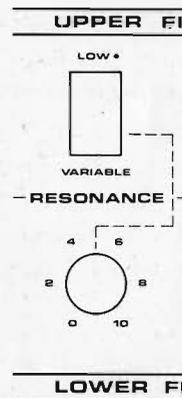
RESONANCE always determines the amount of resonance, or “Q” on the Lower Filter. It also determines the amount of Upper Filter resonance when the LOW-VARIABLE switch is to VARIABLE, for both 12dB and 24dB modes.
