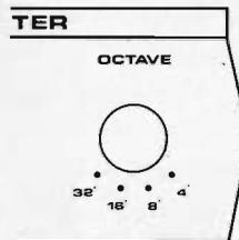
MASTER OCTAVE transposes both oscillators in octave steps. The footage designations 32' 16' 8' 4' are adapted from pipe organ terminology; at the 8' position, the C one octave from the bottom of the keyboard will sound middle C. (This is always true for Oscillator A, and is true of Oscillator B when its OCTAVE/RANGE switch is in the UNISON position, and INTERVAL is set to zero.) The MASTER OCTAVE switch extends the pitch span of the Spirit well beyond its three octave keyboard.
