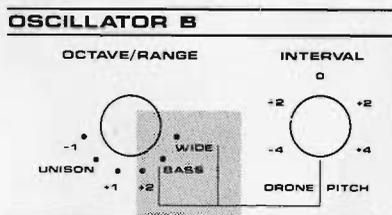
OSCILLATOR B INTERVAL transposes Osc B up or down as much as a perfect fifth when the adjacent OCTAVE/RANGE is in one of the first four “octave step” positions. The center zero position causes no transposition; slight deviations from center create the slight mistuning between the oscillators that adds warmth and fatness to the sound.
