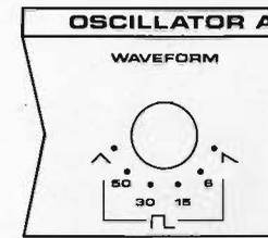
OSCILLATOR A WAVEFORM selects triangle, rectangular, and sawtooth waveforms from left-to-right as panel graphics indicate. The percentage duty cycle of each rectangular waveform is indicated by number within the bracket. Duty cycle is the percentage of time during a single cycle that the rectangular waveform stays at a high level. For instance, the selection marked "50" is a 50% duty cycle rectangular wave, known as a "square wave."
