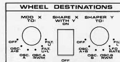
WHEEL DESTINATIONS are the places that modulation signals are routed after passing through the MOD X and SHAPER Y wheels.
