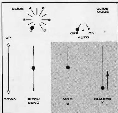
**YOU LEARNED:** MOD X wheel determines the maximum depth of modulation routed to MOD X TO: switch. SHAPE X WITH Y switch shapes within that maximum.
