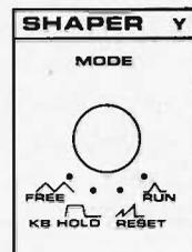
The MODE switch determines how the Shaper will respond to gates:
