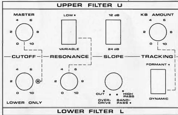
The filters in the FILTER/ADSR path may be used to create various filter responses. The Upper Filter is a lowpass resonant filter with choice of 12dB or 24dB cutoff slope. The Lower Filter may be configured to be either a Parametric Boost or Highpass resonant filter.
