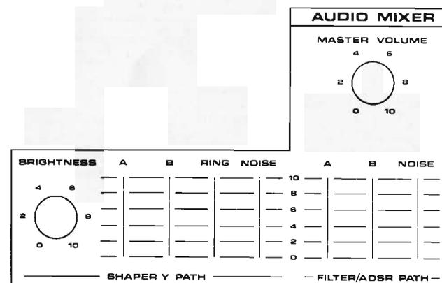
Controls in this section let you combine the sound sources available to both audio signal paths, adjust brightness in the SHAPER Y PATH, and adjust overall volume of both paths.
