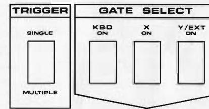
Timing signals (gates) initiate the action of the envelope generators and the Shaper. These signals may be caused by the performer, using the keyboard, be generated by “clock” circuitry that comprises a part of LFO circuits, or be introduced to the Spirit from external sources, or the Shaper.
