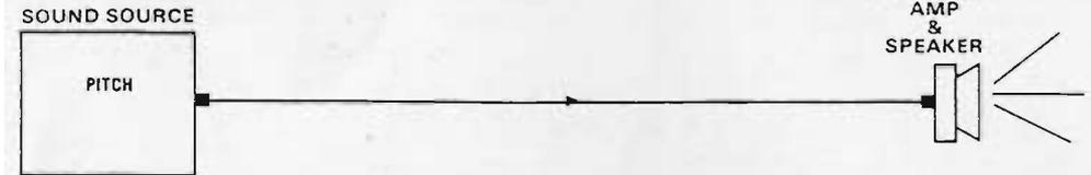
The sound produced by this most basic of "patches" is not interesting. The sound properties are static — they don't change. Now let's insert the timbre and loudness modifiers between the sound source and the speaker:
