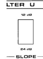
Makes Upper Filter slope = 24 dB/Octave.
