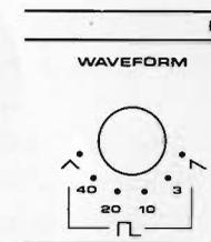
OSCILLATOR B WAVEFORM selects Oscillator B waveforms and functions like its Oscillator A counterpart. Note, however, that the rectangular widths, or selection of duty cycles is not the same as for Oscillator A. This feature provides more tone color possibilities.
