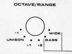
OSCILLATOR B OCTAVE/RANGE is used to tune Osc B relative to Osc A. The first four switch positions provide tuning in octave steps. Osc B can be tuned to the same octave (UNISON), one octave lower or higher, or two octaves higher than Osc A.
