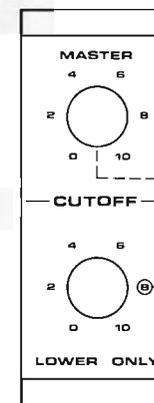
MASTER CUTOFF moves the cutoff frequencies of all filter sections through the audio range. The cutoff frequency of the Lower Filter coincides with that of the Upper Filter when the LOWER ONLY control is set to 8.
